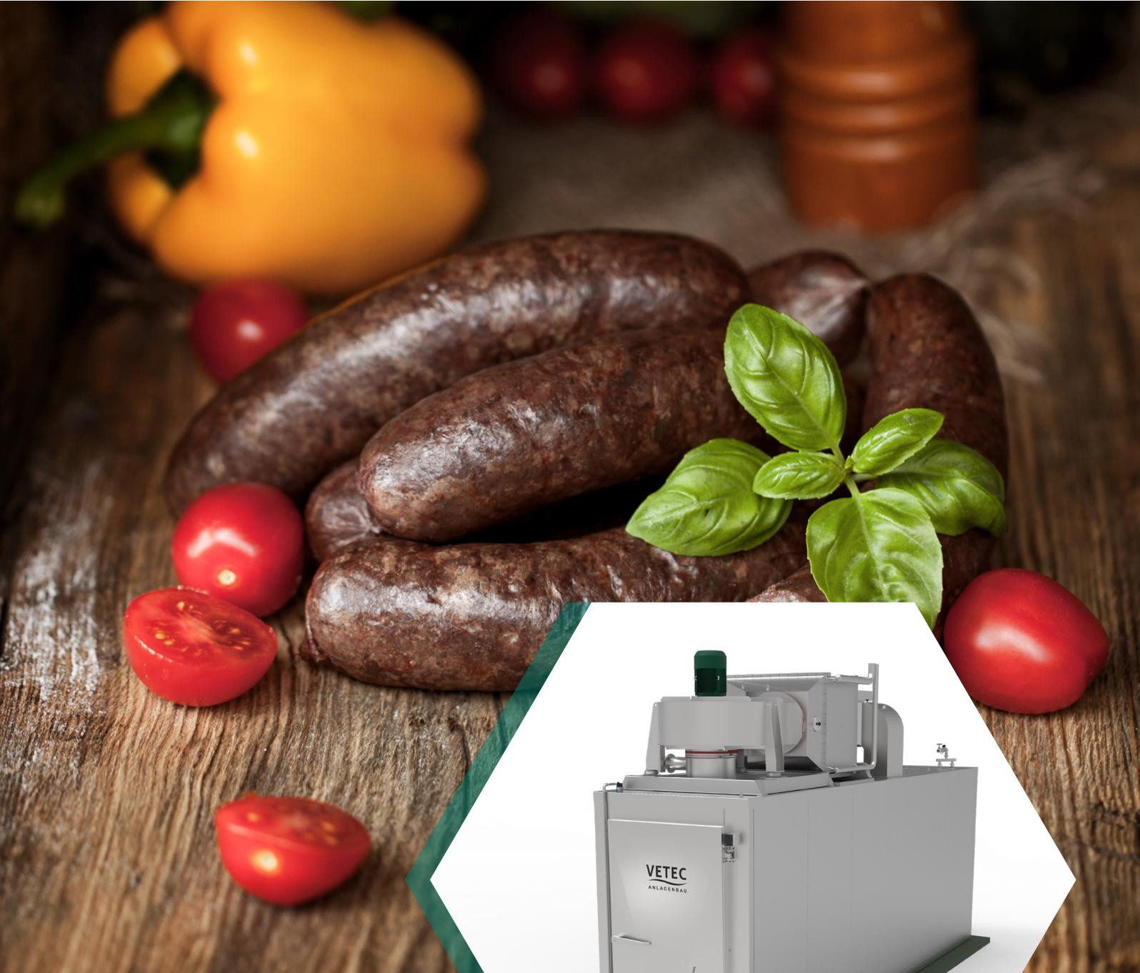
The **AEROMAT<sup>COOL</sup>** is the perfect solution for combined water/air cooling. Sausage, meat products and fish, as well as other suitable foods, are cooled to a certain core temperature with shower water and air immediately after the heat treatment. The product can be packed immediately.
